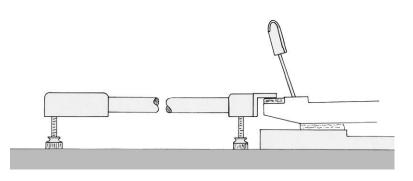
the action in the piano, using a 7/8" gauge held against the underside of the strings, playing the sample keys so the hammers bump the gauge. Fine adjust jig height as needed, and you are ready to install/adjust all dampers.
